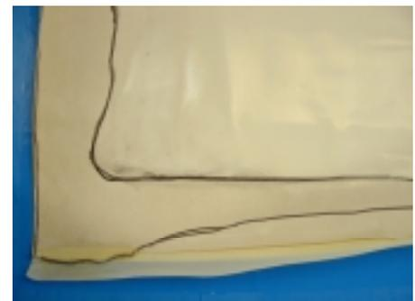
Figures 1 to 4 clearly show that CMRT-produced glue lines are more variable and have a significantly larger width than glue lines produced by the AMEC technique. Note that a significant proportion of membrane area is lost due to the wider glue lines in CMRT-constructed membranes – area that in a FILMTEC element is available, making the element more productive.
