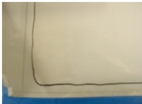
Figure 4. Manual glue line (CMRT construction) (detail)
