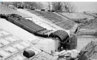
Because of its robust construction, B-series pumps are sometimes used for dewatering in construction site. Compact shape allows high portability comparing against the horizontal pump which requires a firm installation foundation work. In such case, some pump parts are changed its material into harder materials.
