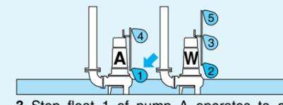
3 Stop float 1 of pump A operates to end water discharge. At the same time, start float 3 of pump W becomes ready for operation.
