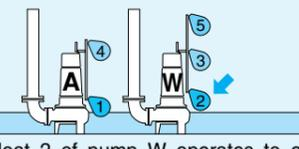
3 Stop float 2 of pump W operates to end water discharge. At this time, alternation start float 3 of pump W rests for one discharge operation.
